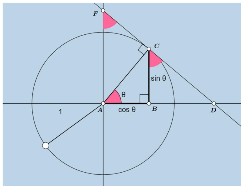
Figure 3: Geometric Construction of Trig Functions from Unit Circle
