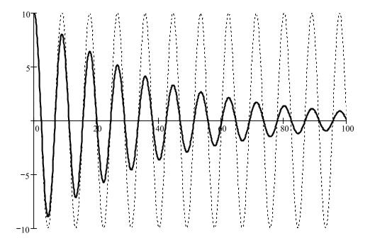
Figure 3. Example of damped motion, with undamped (dotted) motion for same initial displacement.
