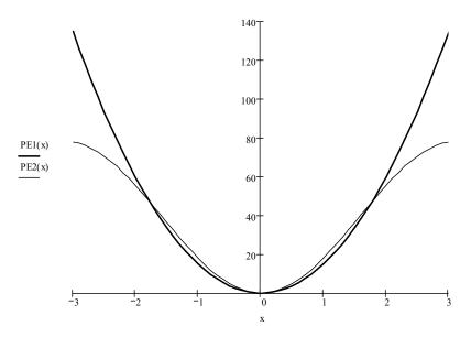
Figure 1 The potential-energy well; thick line is spring-mass, thin line is pendulum.
