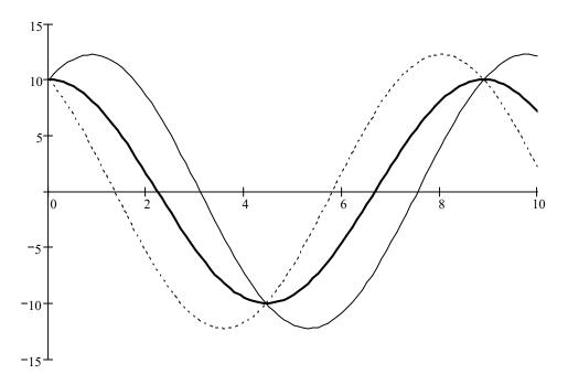
Figure 2. Example solution from Eq(7) for positive (thin line), negative (dotted line), and zero (thick line) initial velocity. Initial displacement 10 units for all three. Positive and negative magnitudes equal. No damping. Note increased amplitude for nonzero initial velocity cases, and the "phase angle" (shifting) effect.
