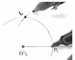
**Step 6:** Connect **m** to **L** using a straight edge.
