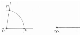
**Step 3:** Using the same settings for your compass as step 2, place the point of the compass on point *m* on your line from step 1.
