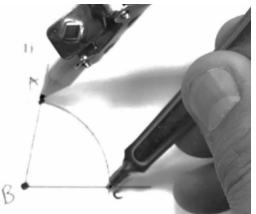
Step 5: USING THE SAME COMPASS SETTINGS AS STEP 4, place the point of the compass on *n*.
