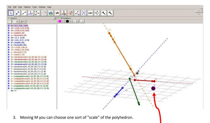
One point is particularly interesting, it is when the polyhedron reduces to **one single point**, and beyond, reverses itself. This point may be considered as sort of "Centroid" of the system of 4 forces...
